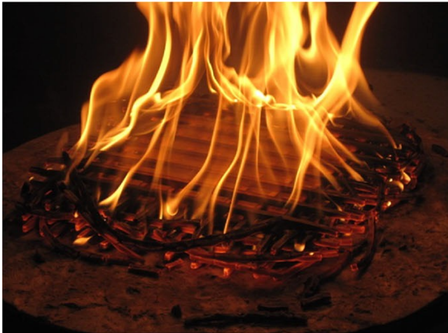
Under-ventilated wood crib (flame stabilized on the outer edge of the crib, \phi > 1 )
