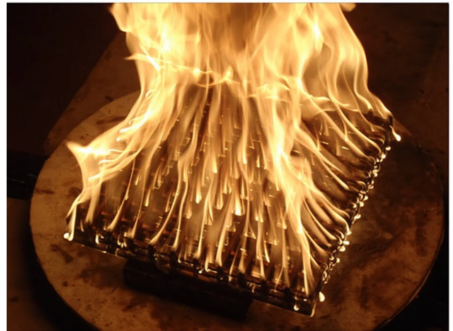
Over-ventilated wood crib (flames stabilized around individual sticks, \phi < 1 )
