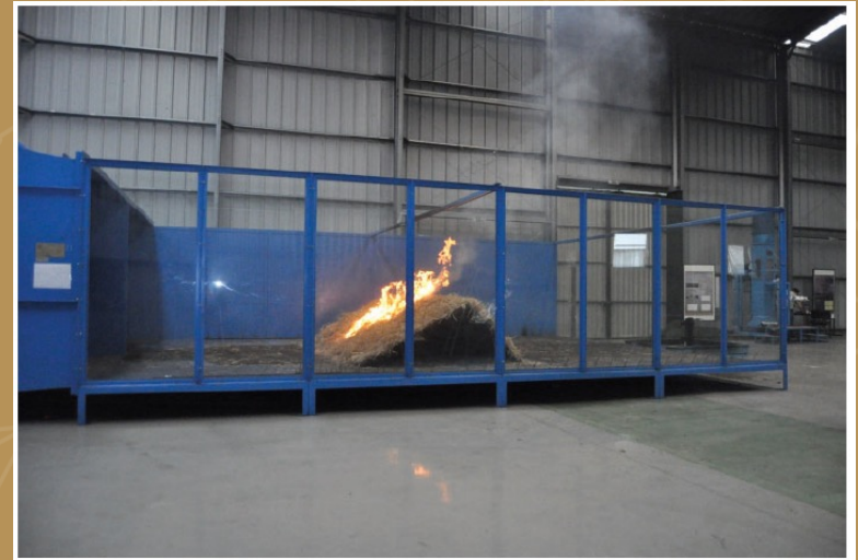
Fig. 2. General view of the combustion wind tunnel of the Forest Fire Research Laboratory of the University of Coimbra with the model of the two-dimensional hill. The length of the working section is 8 m and its width is 6 m. Maximum flow velocity is 8 \text{ m s}^{-1} .
