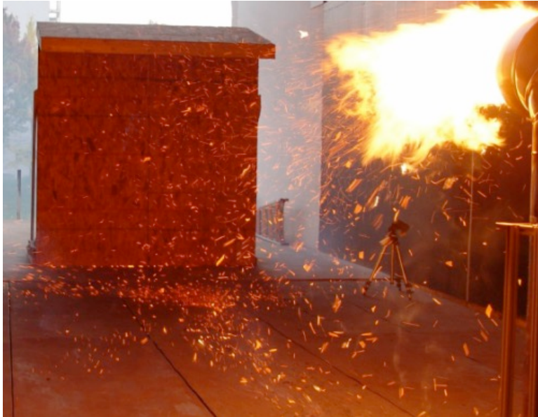
A typical experiment with the NIST Dragon in BRI's FRWTF
