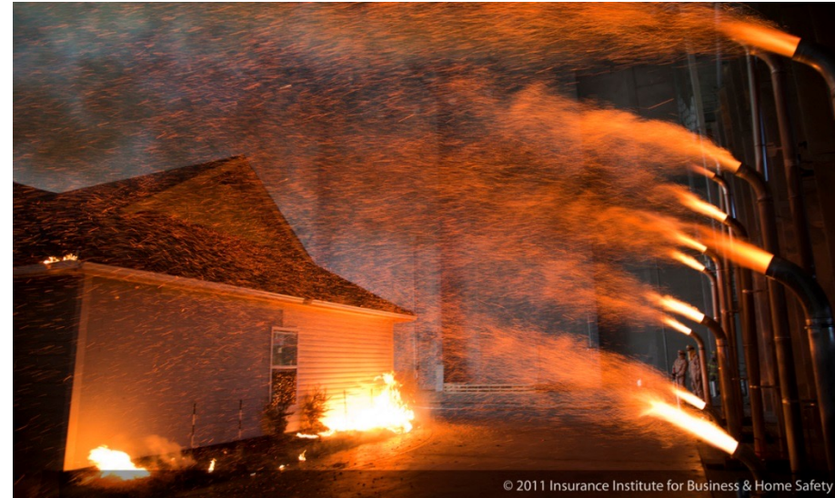
“Ember storm” produced in the IBHS research facility
